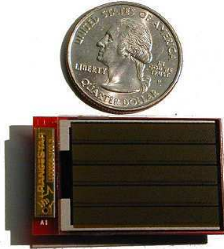
Fig. 1.5 PicoBeacon from UC Berkeley.
