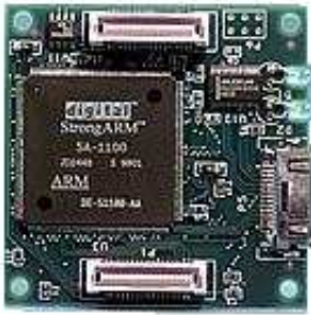
(a) The WINS processor board
